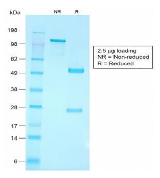
Integrity of the purified antibody AE00109 under non-reduced and reduced conditions, showing intact IgG at around 130kDa (NR) and intact heavy and light chains at 50kDa and 25kDa resp. (R).
